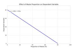
The regression analysis shows a significant negative relationship between the proportion of waste material and the compressive strength of the concrete ( $\beta$  = -0.5, p < 0.001), indicating that higher proportions of waste material tend to reduce the compressive strength. However, this relationship varies depending on the type of waste material used, as demonstrated by the superior performance of geopolymer concrete.
