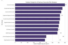
The environmental impact evaluation reveals that geopolymer concrete mixes (fly ash and slag) have the lowest greenhouse gasoline emissions, electricity consumption, and waste generation. additionally show off the smallest carbon footprints, highlighting their environmental benefits in comparison to standard and different waste-included construction substances.
