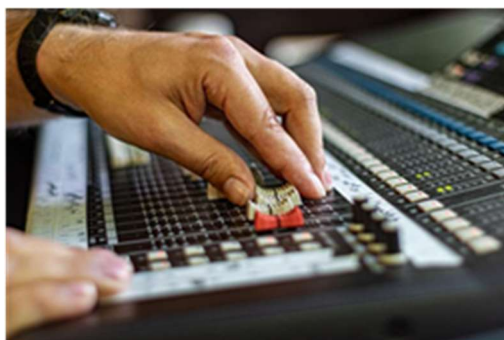
Figure 13: Mechanical tools of acousmatic interpretation: Faders and potentiometers
