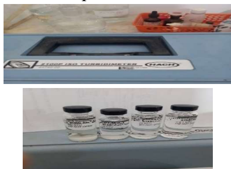
Figure (26) Turbidity Meter and Calibration Process
