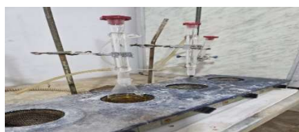
Image (27) Method for Titrating Chemical and Biochemical Oxygen
